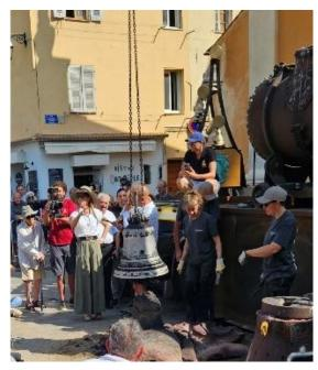
The still-steaming mould had its core slowly pulled out by the crane mounted on the lorry and the remaining assembly was carefully rotated through 180 degrees and left hanging six feet in the air. There then followed some very aggressive use of wooden mallets to separate the outer parts of the case (the cope), which fell to the ground along with most of the casting sand.
